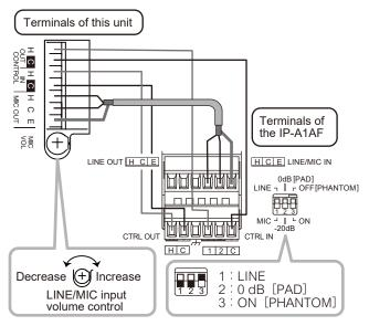
Power is supplied to the unit by a phantom power supply (9-26 V DC).Before connecting the unit to the IP-A1AF, be sure that the Interface's DIP switch is set as shown in the figure above.
